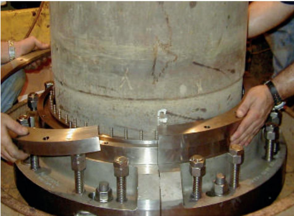
*Big is no problem. A 24 inch split seal being installed on a turbine for hydroelectric power generation.*
