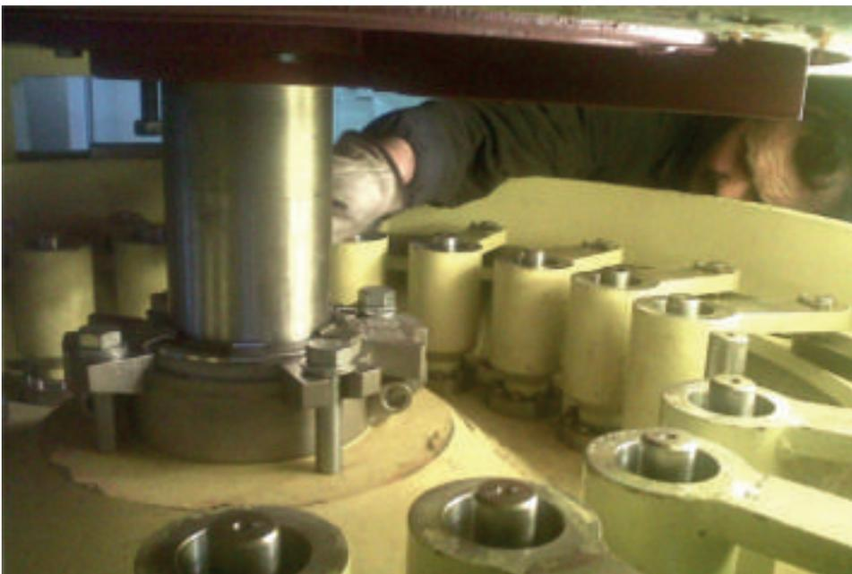
*Kaplan turbine sealing. A maintenance-free sealing system in which split seals provide operators of small hydro power plants peace of mind with reliable and maintenance friendly sealing.*
