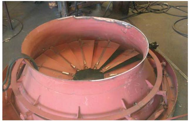
*These are the inlet guide vanes from a forced draft fan that suffered a premature failure. The guide vanes were not properly attached to the fan plenum and fell on the impeller. The picture is of the vanes and inlet cone being repaired.*
