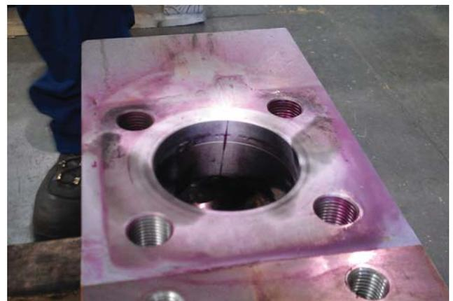
*Picture of the head of a reciprocating pump that suffered a fracture. Dye penetrant was used to help define the severity of the crack. The red line is the dye leaching out from the crack. The crack was discovered when the pump started leaking.*
