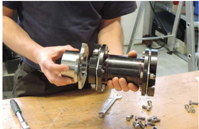
An assembly technician checks the fit of a new LPAI disc coupling for a centrifugal pumping application. The LPAI drives the disc packs by pure face friction, within an easily removable spacer cartridge.
