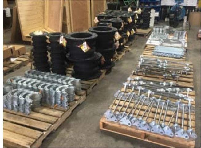
*Style 232 & 233 open and filled arch expansion joints w/limit rods.*
